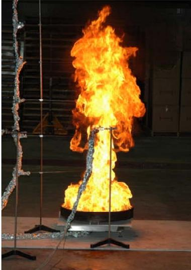
From the above results, it is observed that the 1-meter values are consistent and compare favorably to the actual measured values. The 0.50 results do not show as much accuracy and this can be attributed to the fact that the calculated results and measured results are less than a flame diameter away from the flame axis. The equation can be effectively utilized with the values derived from other equations, such as Heat Release
