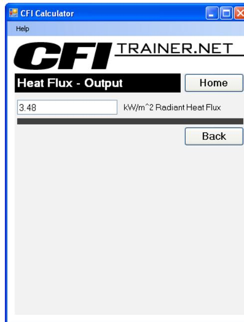
The 2005 Fire Research Laboratory experiment can again, be utilized as an example of the practical application of the heat flux calculation. Recall that the experiment involved burning approximately 3.79 liters (1 gallon) of gasoline in a pan measuring approximately 0.55 meters (22 inches) in diameter and heat flux gauges were
