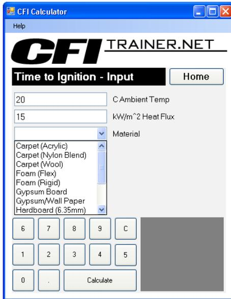
While there are other variations of the Time to Ignition calculations, including an alternative formula for thin fuels and an alternative variable that account for heat loss by the target fuel<sup>19</sup>, this calculation and the CFI Calculator tool can appropriately be utilized to give a reasonable estimation for use by the field investigator.
