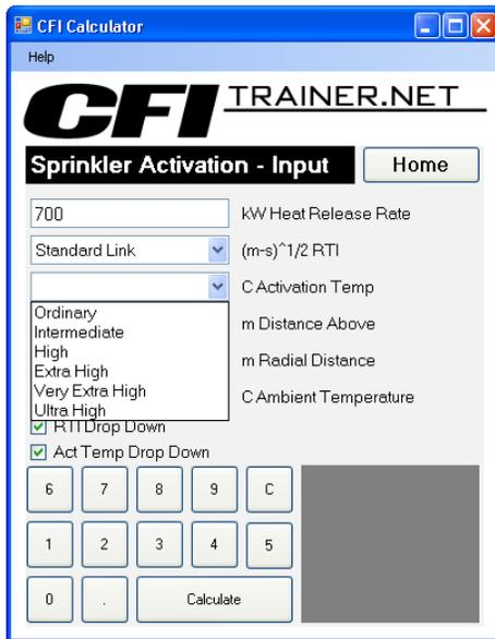
While it is best to utilize this calculation with the specific information on the sprinkler device in question, estimated results can be obtained utilizing the drop down menus and the input data contained within the program. As with the other calculations contained in the CFI Calculator, it is advisable to run multiple iterations of the Sprinkler Activation calculation to derive results that define a reasonable analysis of what might have occurred and allow you to “bind” the problem.
